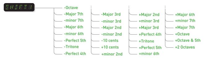
Shift 2: Selects the 2nd voice interval, from an octave down to two octaves up. Can be set to Off if no 2nd voice is desired.
