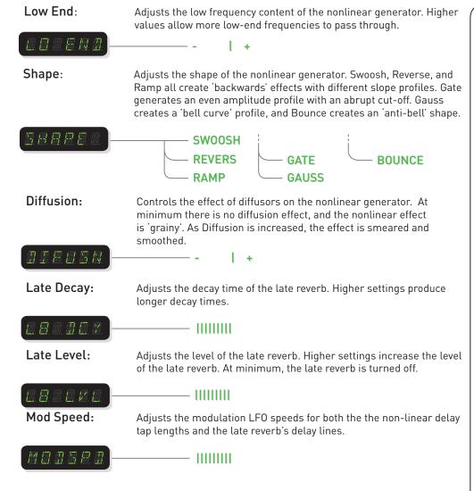
**KNOB FUNCTIONS:** In Nonlinear, two of the knobs assume different controls than the other reverb machines.
